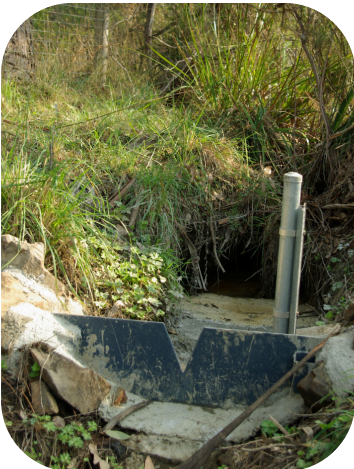
V-notch weir, measuring flow rate from water level data.
