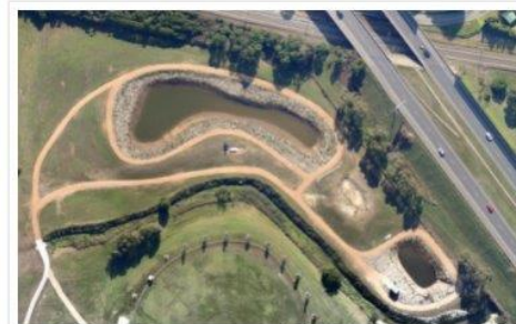
Stormwater harvesting at Sweeney Reserve. Anti-clockwise: sediment catchment pond for water coming from Melbourne Water's drains, raingarden removing gross pollutants, storage pond at the top.
