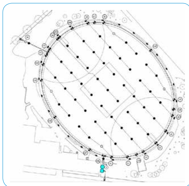
Figure 14: Best Practice irrigation design for a sports ground
