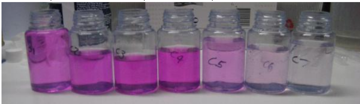
Plate 2: Example of Final Rinse Time Sequence with Phenolphthalein Indicator Added to Each Bottle
