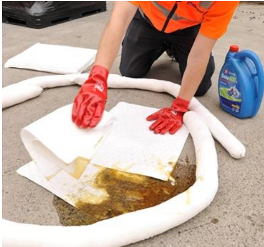
Figure 7.4. Containment and cleanup of a spill.
