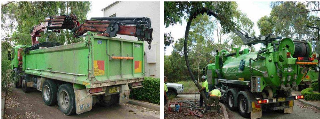
Figure 21 Whichever cleaning method Council chooses, or the cleaning contractor uses, its important to note that the trucks used are fairly large, so driveways and parking areas for them are a good idea. Whilst not required everywhere, it avoids rutting if you have at least a semi-formalised access.
