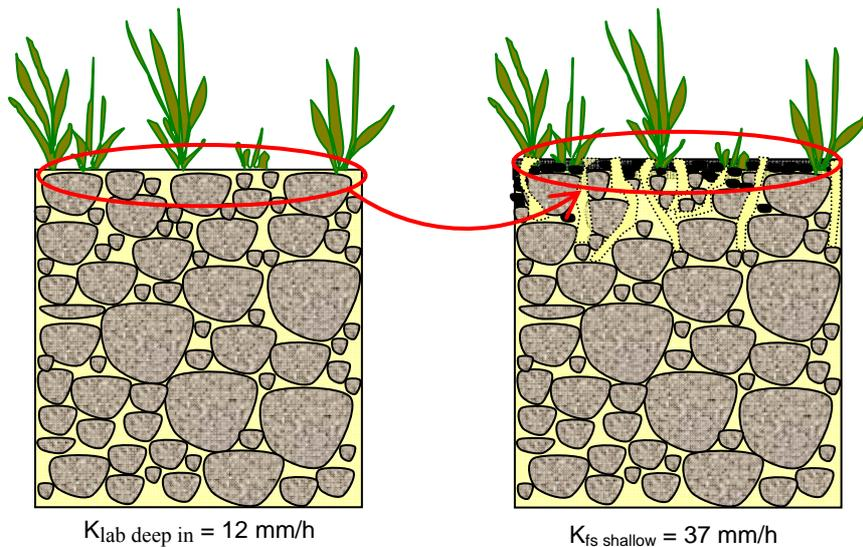
Figure 9 : Schematic representation of the evolution of the behaviour of biofilters with low initial K
