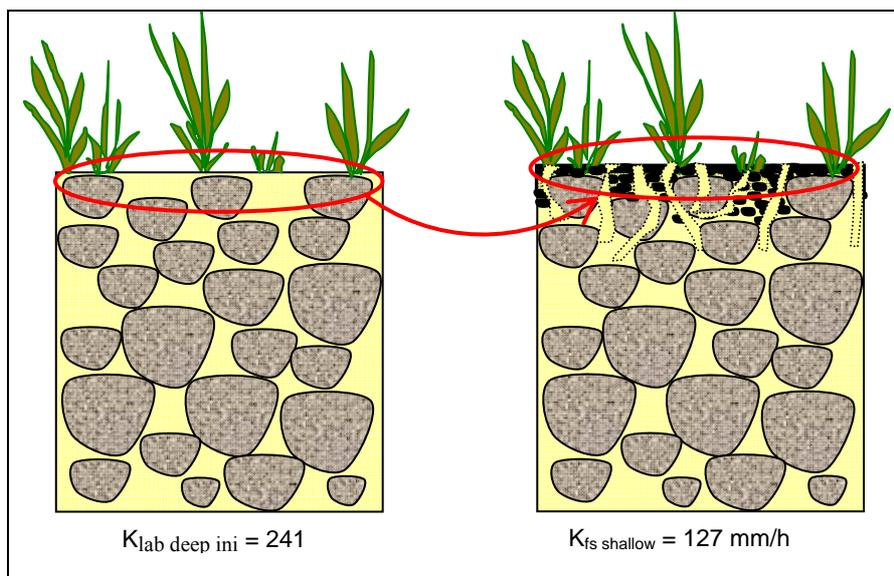
Figure 8 : Schematic representation of the evolution of the behaviour of biofilters with high initial K
