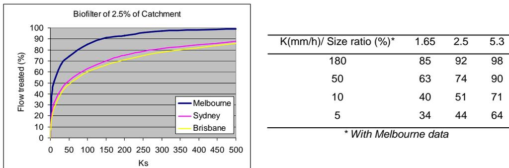
Figure 3: Influence of the ratio biofilter/catchment size and of the  $K_{fs}$  on the ‘hydrologic effectiveness’
