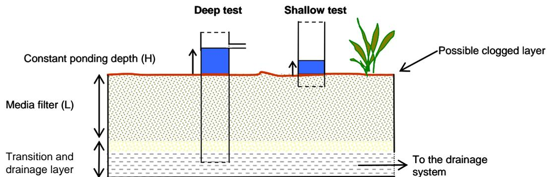
Figure 2: Sketch of a biofilter with the deep ring and the shallow ring
