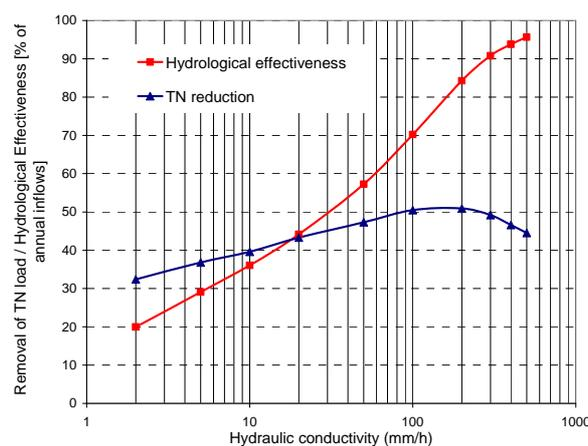
Figure 1 : Evolution of Hydrological effectiveness and TN reduction vs. Hydraulic conductivity
