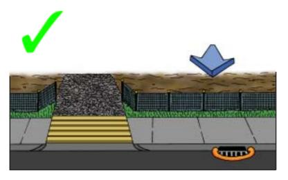
Putting crushed rock on the access point of your site is a good way to prevent damage and provide a dry access point for vehicles. Where possible park vehicles off site.
