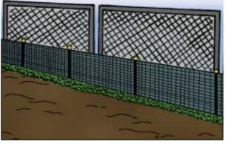
Remember to install a sediment control fence prior to installation of the temporary fence.
