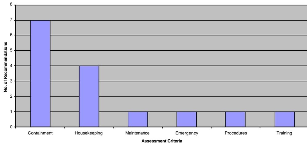
The main area for improvements in this industry was containment and housekeeping. The industry may benefit from the use of bund pallets to improve storage of lubricating oils and the installation of drip trays under the equipment to contain any oils used during the cutting process. Stormwater management performance could also be improved by obtaining appropriate spill kits.
