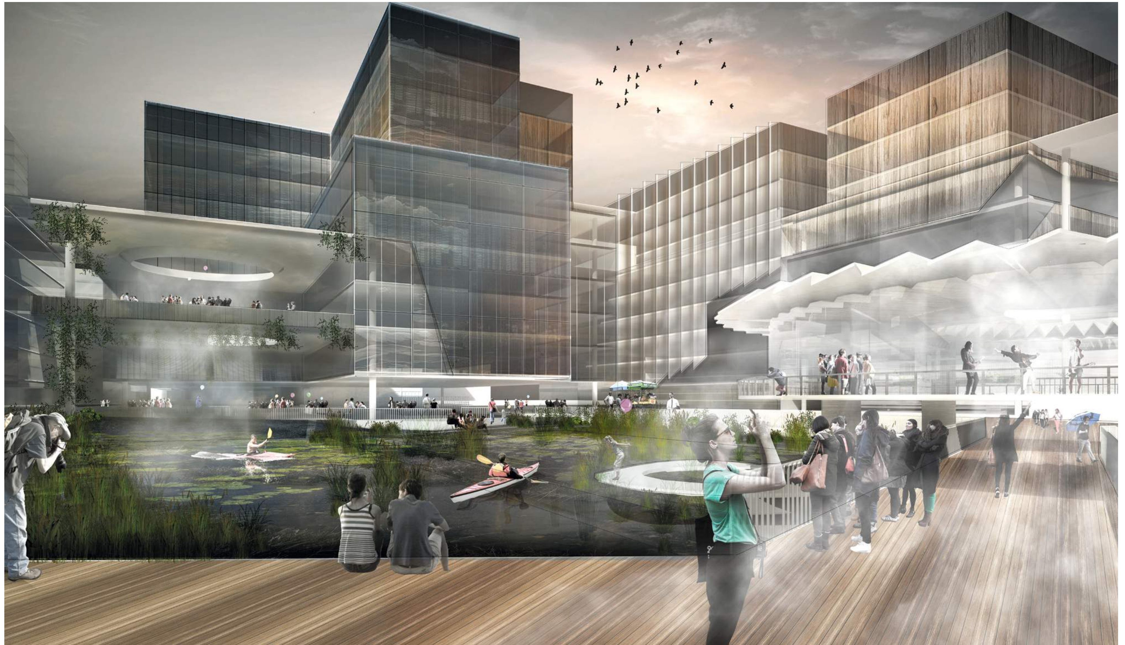
An urban square within the new development zone acts as a storage basin for excess stormwater.
