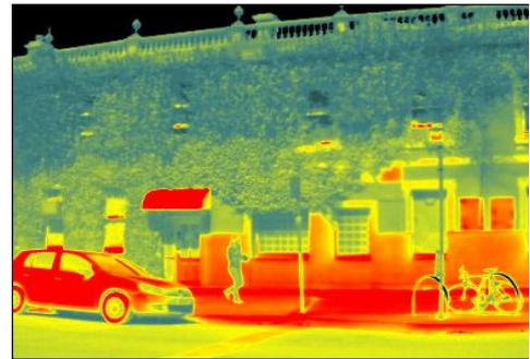
Figure 7: Green facade in inner-Melbourne during the day. Blue indicates lower temperatures and red, higher temperatures (image taken with a thermal camera. Photo: R. Harris)
