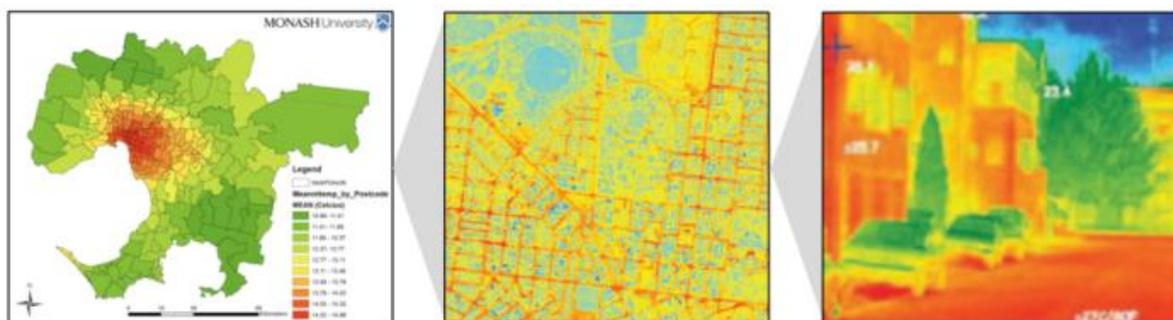
Figure 4: Urban surface temperatures measured at different scales (from left to right): Greater Melbourne using satellite data [1]; at the neighbourhood scale using airborne thermal imagery; and at the street-scale using a thermal camera [2]. Red indicates high temperatures, green and blue are lower temperatures. [3]. Street scale (image from urban-climate-energy.com) Note temperature colouration scale varies between images)
